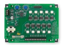
The **SERIES DCT500A** Low Cost Timer Controller is designed to provide continuous or on-demand cleaning for receivers and pulse jet systems. It is available in either 4, 6, or 10 channels, and each unit is the same size, minimizing enclosure space and reducing overall system installation cost. For added safety, the control circuitry including the control inputs are isolated from the line voltage.
