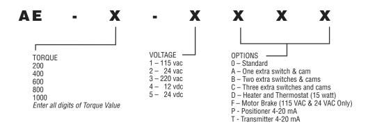
Note: AE will always be the first two characters of the part number, all digits from torque value must be entered into part number (i.e. 400, 1000 etc.) Only use one digit for voltage depiction (i.e. 1-5). For the options listing you may use more than one character, up to three, (i.e. 0, AD or BD etc.)
