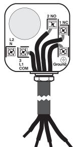
GAO Low or High Gas Switch (Operating state shown as a high limit). As pressure rises above set point, 1 NC opens, 2 NO closes, Neon light ON. As pressure falls below set point, switch resets: 1 NC closes and 2 NO opens, Neon light off.
