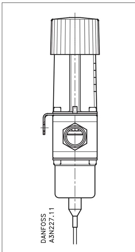
The valves can be installed in any position. An arrow on the valve body indicates the direction of flow.
