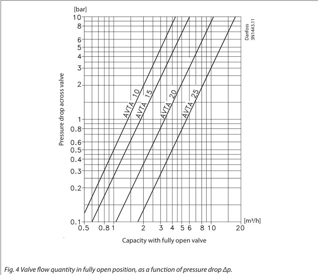
Fig. 4 Valve flow quantity in fully open position, as a function of pressure drop  $\Delta p$ .
