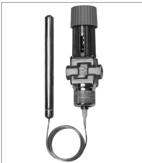
AVTA thermo. operated water valves are widely used for temperature regulation in many different machines and installations where cooling is required. AVTA cooling water valves always open to admit flow on rising sensor temperature.
