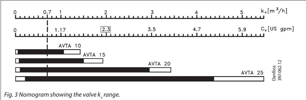
Fig. 3 Nomogram showing the valve  $k_v$  range.
