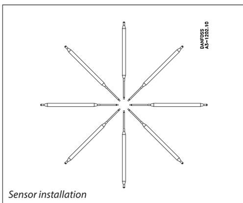
The charge consists of active carbon and CO<sub>2</sub> which is adsorbed on falling sensor temperature, thereby producing a pressure change in the element.
