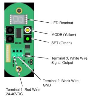
**STEP 4** Measure the output signal between pin 3 (white signal output wire) and pin 2 (black ground/shield wire). It should match the milliamp reading found in Step 2. If you do not read between 2 and 22mA milliamps, then you have an issue with your cable and/or plugs. Ohm check the cabling back to the control panel.
