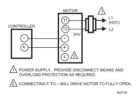
Fig. 5. Typical system wiring.
