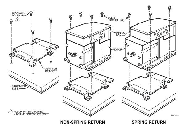
Fig. 3. Mounting the motor with an adapter bracket.
