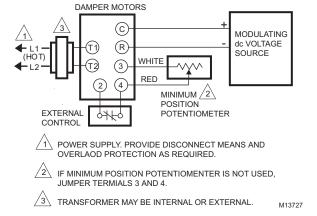
Fig. 7. M7685 Typical application wiring.
