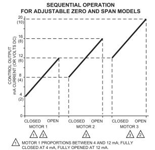
MOTOR 2 PROPORTIONS BETWEEN 8 AND 16 mA; FULLY CLOSED AT 8 mA, FULLY OPENED AT 16 mA.
