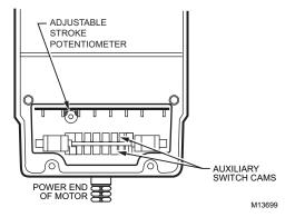
Fig. 9. Stroke adjustment setup
