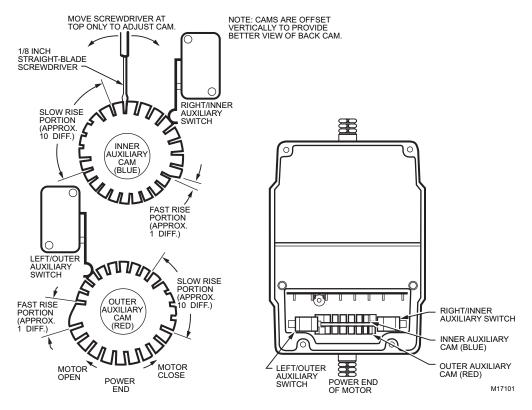
Fig. 12. Auxiliary switch adjustment.
