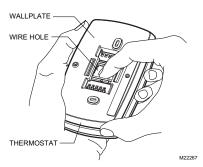
Fig. 2. Separate wallplate from thermostat.
