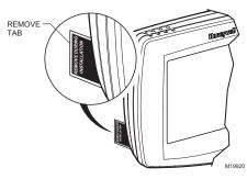
Fig. 23. Remove tab labeled REMOVE from thermostat back.
