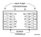
Fig. 4. Terminal identifications for system type.
