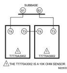
Fig. 19. Wiring two T7770A3002 (10K ohm) Sensors to provide a temperature averaging network.
