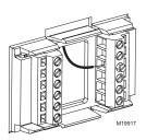
Fig. 5. Insert wires into terminal block.
