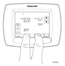
Fig. 26. Entering Installer Setup.
