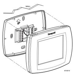
Fig. 25. Mount thermostat to wallplate.
