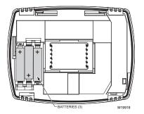
Fig. 22. Installing batteries.
