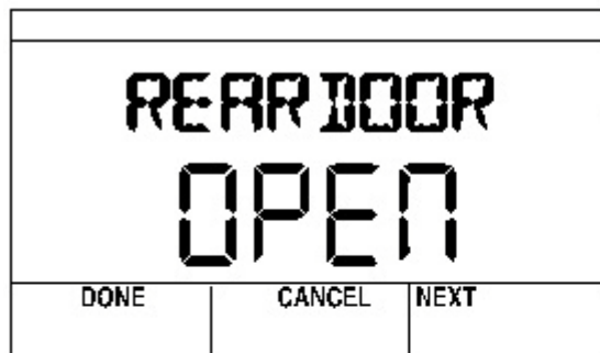
Fig. 36. Sample Contractor parameter display for TR71/TR75 showing enumerated value displays with label instead of numeric value.
