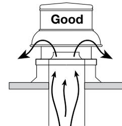
Provide uniform airflow at fan inlet to ensure optimum performance.
