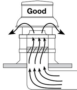
Provide uniform airflow at fan inlet and through the damper to ensure optimum performance. Curb cap should be three wheel diameters from the radius. Use turning vanes in duct when possible.
