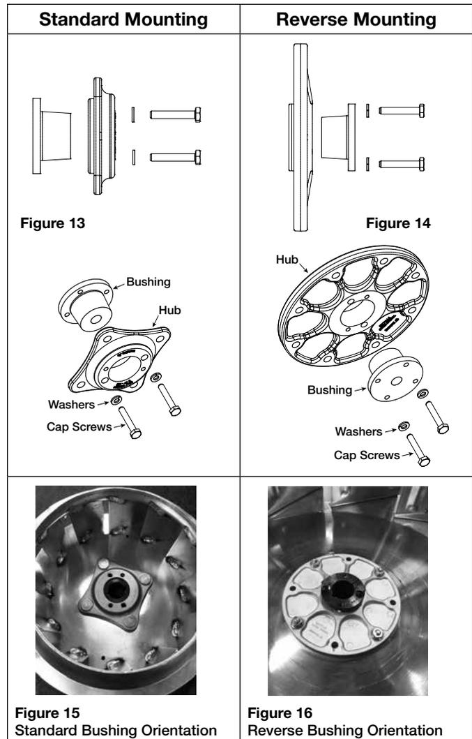
3. **Standard Mounting:** Take the two socket head cap screws that were removed and install them into the visibly threaded holes on the wheel hub.
