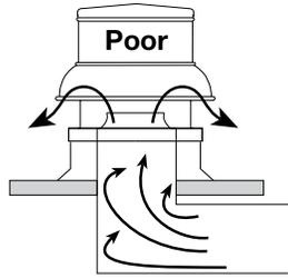
Avoid sharp turns or entrance conditions which cause uneven flow. Use turning vanes in elbows to reduce adverse effects.
