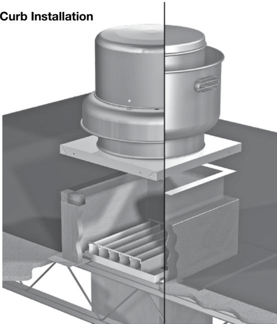
2. If unit is equipped with a backdraft damper, it should be installed now.
