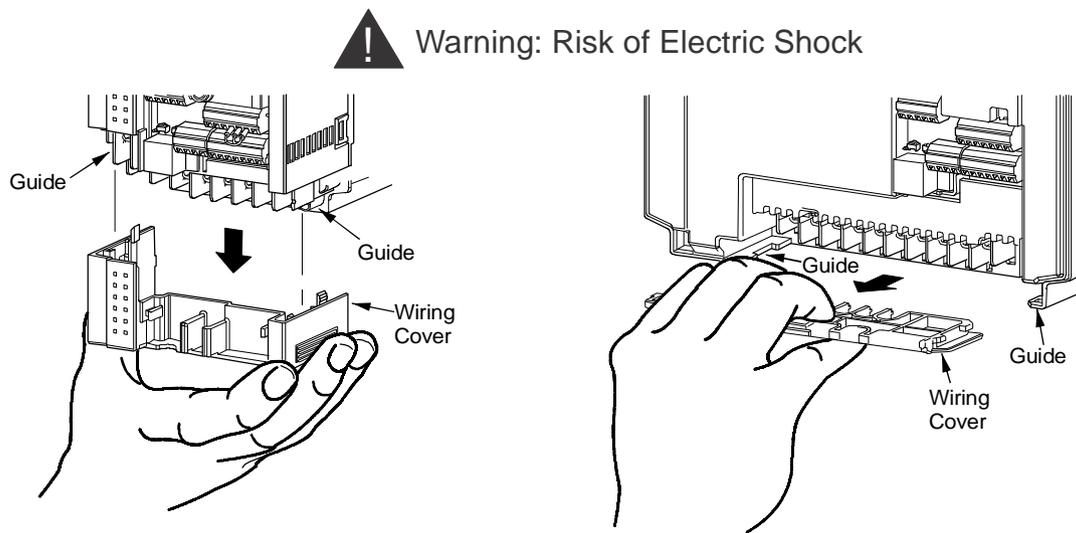
**Figure 10: Remove the High-Voltage Wiring Cover**
