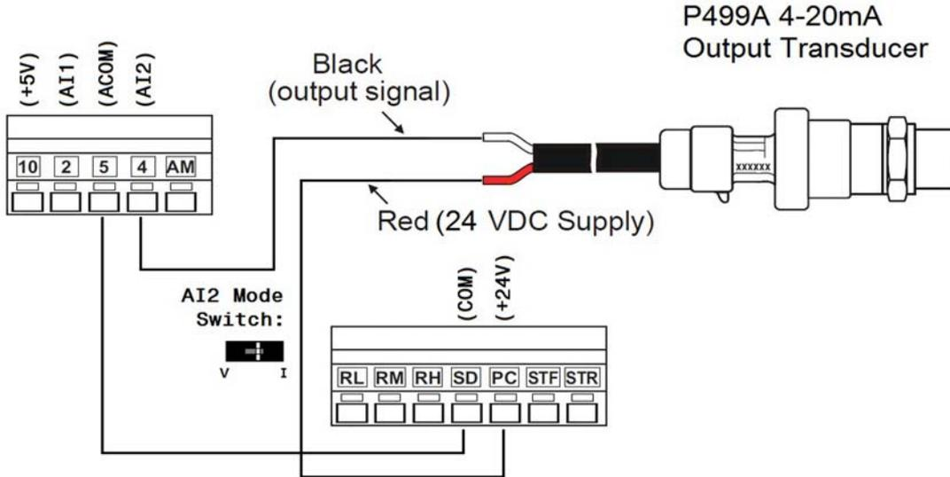
Figure 17: Wiring a 4–20 mA Input Signal Transducer
