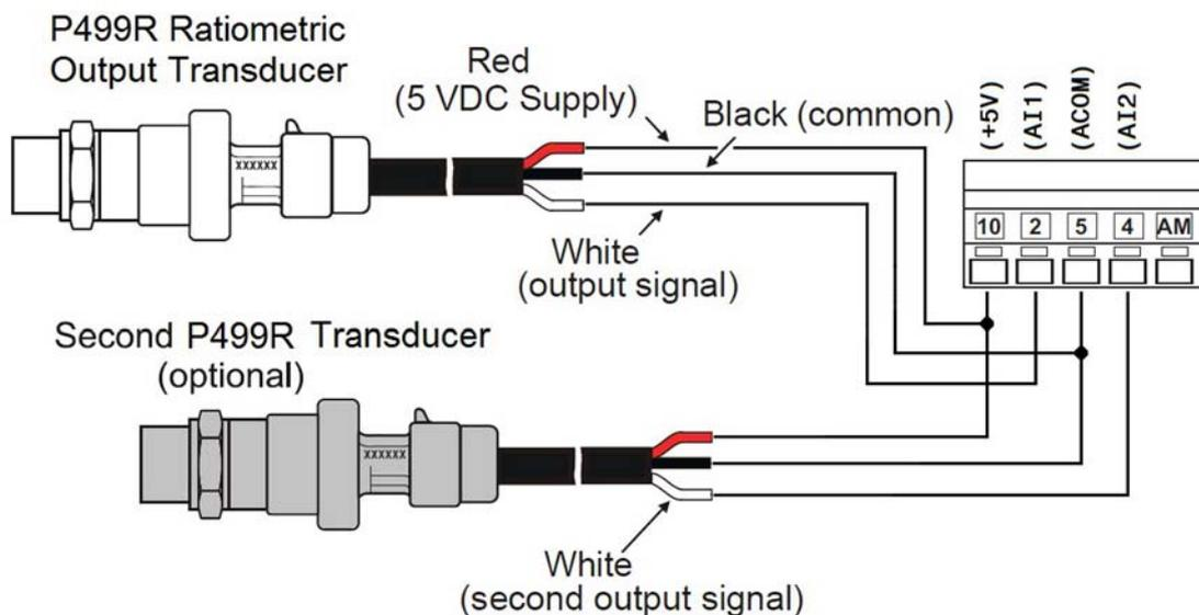
**Figure 15: Wiring 0.5–4.5 VDC Ratiometric Input Signal Transducers**
