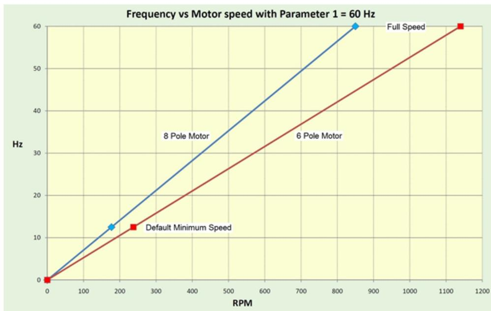
**Figure 19: Frequency and Motor Speed (60 Hz)**
