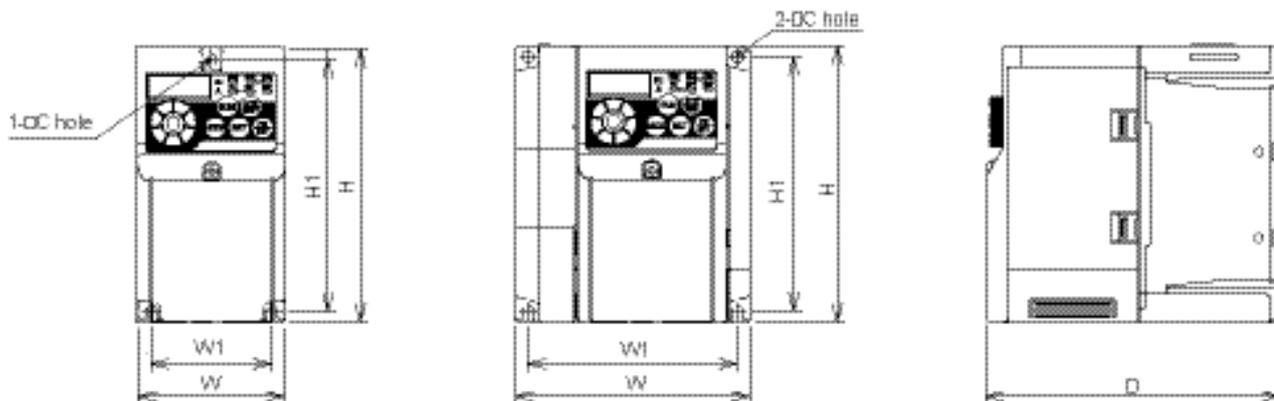
Figure 3: Dimensions for VFD68 Drives, 230–460 VAC Models
