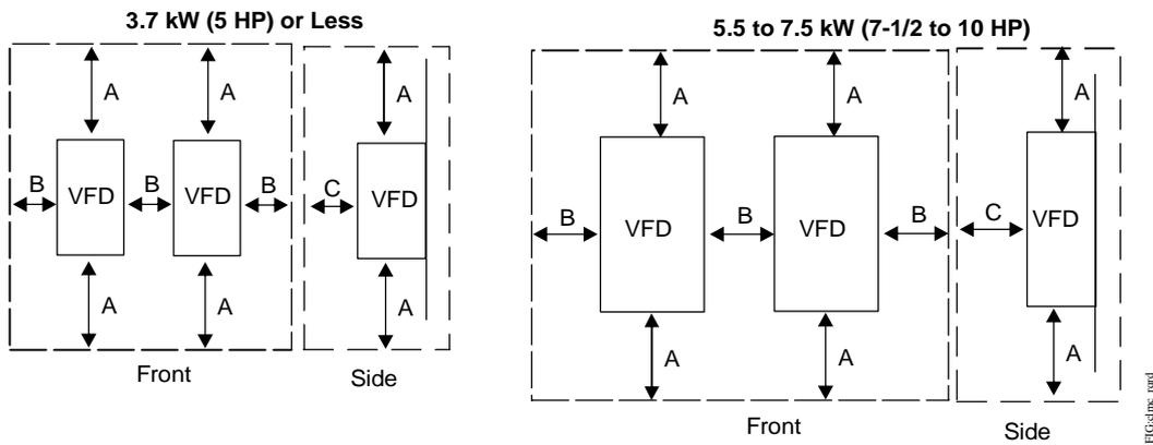
**Figure 7: Required Clearance for Mounting Inside an Enclosure**
