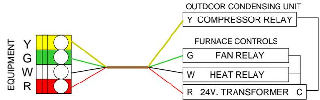
**Transformer** – A separate 24 Volt AC, 40VA Transformer is recommended to power the control panel, thermostats and dampers. Often the transformer on the HVAC unit only has enough power for its own controls. Therefore it is recommended a separate transformer be used to power this panel and the dampers wired to it.
