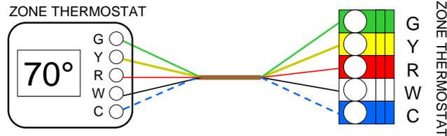
**HVAC Equipment** – The HVAC equipment will follow Wiring Diagram 2 for Single Stage Systems. The MMP2 can also control Heating Only and Cooling Only as well as both Heating and Cooling.
